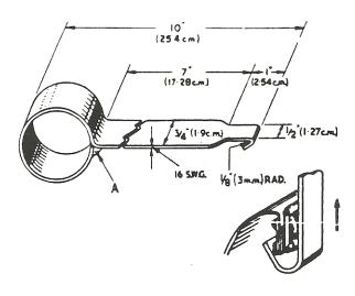
Fig. 12.14. Details of hooked tool for fitting spring clips
